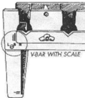
A.) If using LEFT HELICAL FLETCHING, move the NOCK RECEIVER BAR to the LEFT, and the V-BAR to the RIGHT. Use the markings on the frame for "L" or "R" as a guide. These adjustments will have to be made every time you change shaft size (2018, 2117, etc.).
