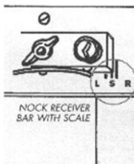
Open the clamps and slide the feathers (vanes) into position until they are even with the mark you placed on the clamps.
