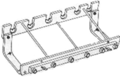
**ASSEMBLY:** Attach both legs to the bottom of the frame with the screws and nuts provided (as shown). Attach the LONG end of the leg to the INSIDE of the keyhole-slotted plate. Attach the SHORT end to the INSIDE of the nock receiver plate. Set the assembled frame and legs on a level surface and tighten screws securely.
